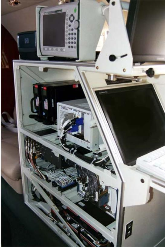
The inside story of the RVA AAFIS (Advanced Automatic Flight Inspection) System as installed by KAAV. The AAFIS incorporates a suite of advanced navigation sensors from Honeywell, Rockwell/Collins, and Ashtec, including differential GPS. It is also integrated into a variety of existing sensor platforms on the aircraft, and has its own dedicated set of antenna systems plus a Chelton System 7 Direction Finding (DF) System - used in the analysis and locating of interfering signals.
