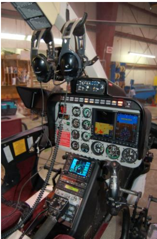
The Garmin G-500H Flight Display System highlights this state-of-the-art ENG cockpit.
