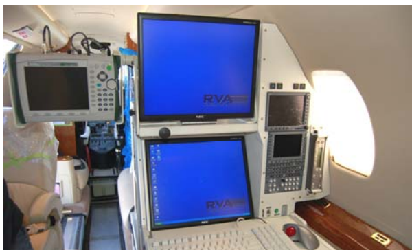
The RVA FIS system as it appears in the cabin. This installation means removal of one cabin seat but still allows the Excel to retain most of its corporate interior for use in its dual purpose of government aircraft and flight inspections.
